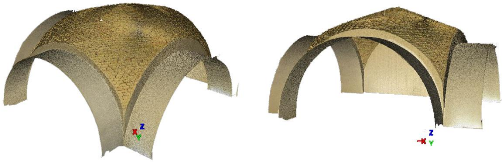
Figure 2: The vault geometry obtained from laser-scanner surveys.
